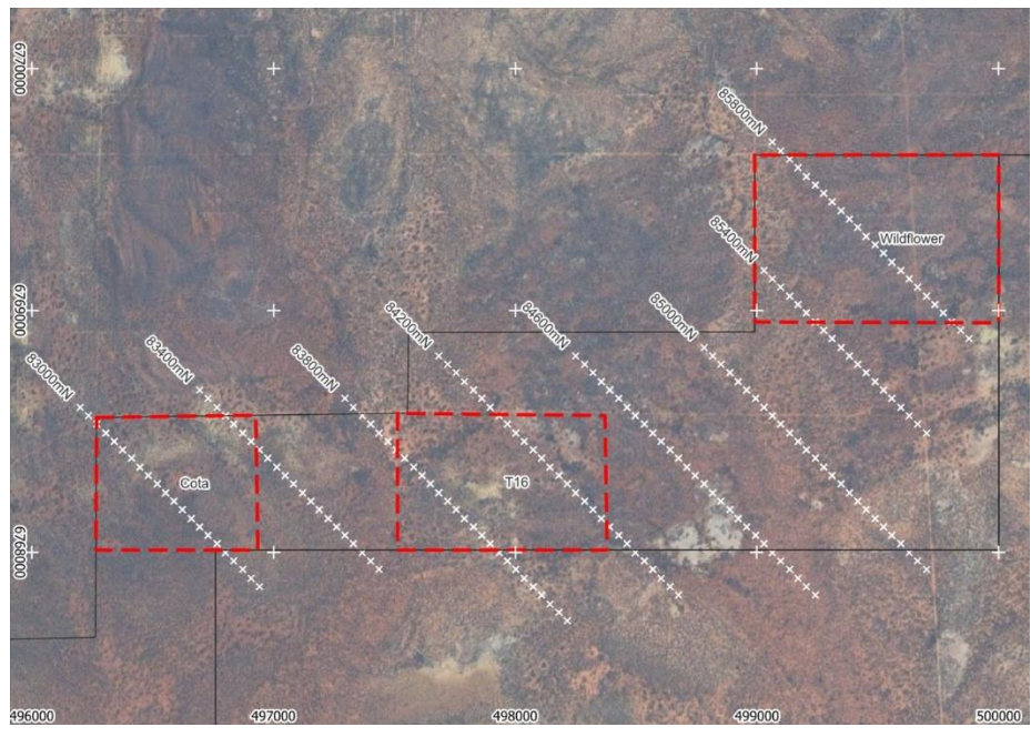
Diagram 10: Location of the induced polarisation (IP) survey stations and lines (shown in white) across Terrain Minerals Wildflower granted tenement E59/2234 and extending into Terrain Minerals adjoining granted exploration tenement E59/2345. The location of the three prospects within exploration tenement E59/2234, namely Wildflower (actual), T16 and Cota are outlined in red also see diagram 9 and 14 (see ASX release 10 November 2025).
