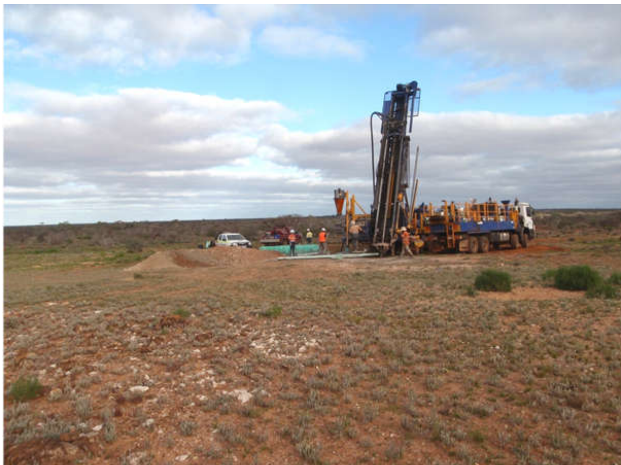
Photograph 3: RMRC 005 and RMRC 006 were drilled at target MG1 from the same drill pad at inclinations of -50 degrees and -60 degrees respectively. Outcropping mafic schist and white calcrete can be seen in the foreground. A schistose mafic unit over 70m thick was intersected here.
