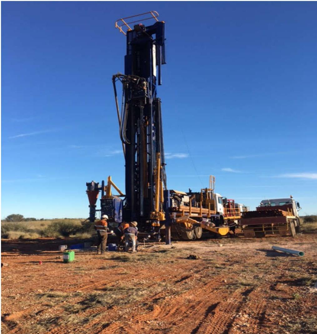
**Picture 1:** Raglan RC drill rig & support vehicles.
