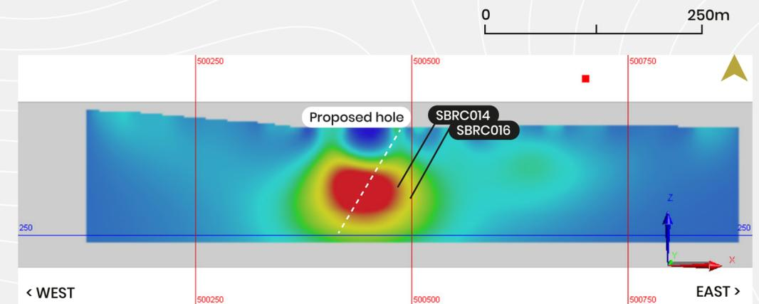
**Diagram above:** Two-dimensional (2D) inversion chargeability sections on 6774000N looking north with Terrain's 2020/21 Monza drill holes superimposed, which appear to have been drilled 50m away from the newly defined IP anomaly. Proposed drillhole shown in white.
