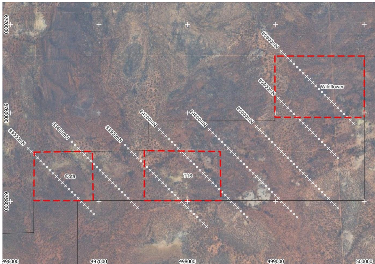
Diagram 4: Location of the induced polarisation (IP) survey stations and lines (shown in white) across Terrain Minerals Wildflower granted tenement E 59/2234 and extending into Terrain Minerals adjoining granted exploration tenement E 59/2345. The location of the three prospects within exploration tenement E 59/2234, namely Wildflower (actual), T16 and Cota are outlined in red.
