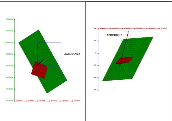
Aztec Dome DHEM Survey - Plan view (left) and section view (right) of drillhole AZRCDD013 and model plates.
