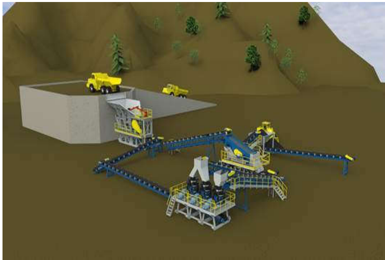
Sepro System: 75t 3 Stage Crushing Circuit
