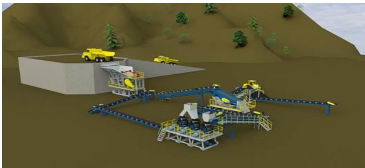
Diagram 7: Sepro Systems 75 tph three stage crushing circuit.
