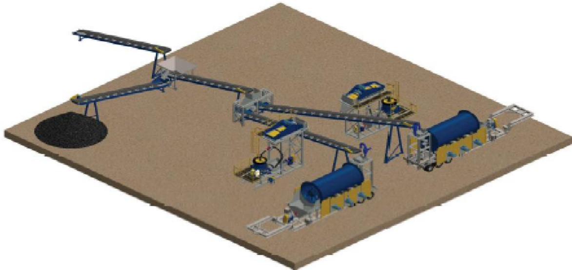
Diagram 8: Sepro Systems 40 tph grinding and gravity plant (dual stream mills and centrifugal concentrators).
