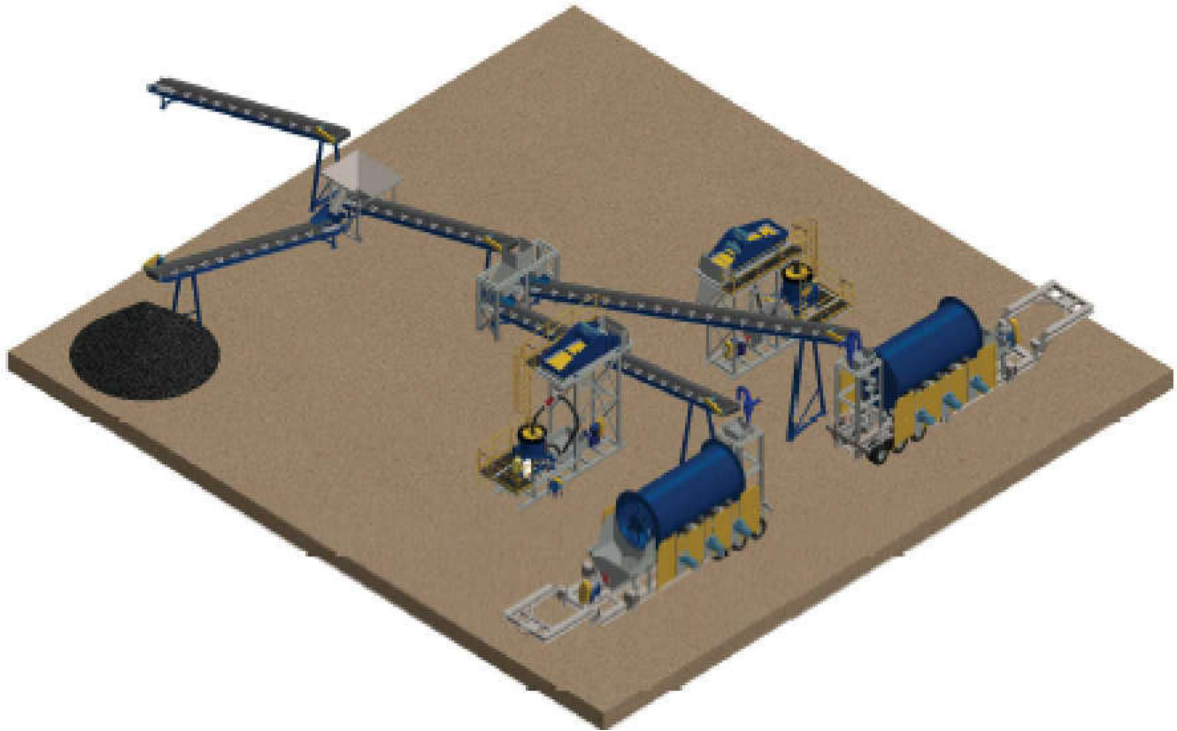
Diagram 8: Sepro Systems 40 tph grinding and gravity plant (dual stream mills and centrifugal concentrators).
