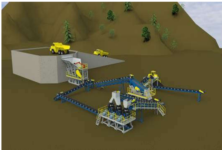
Sepro System: 75t 3 Stage Crushing Circuit
