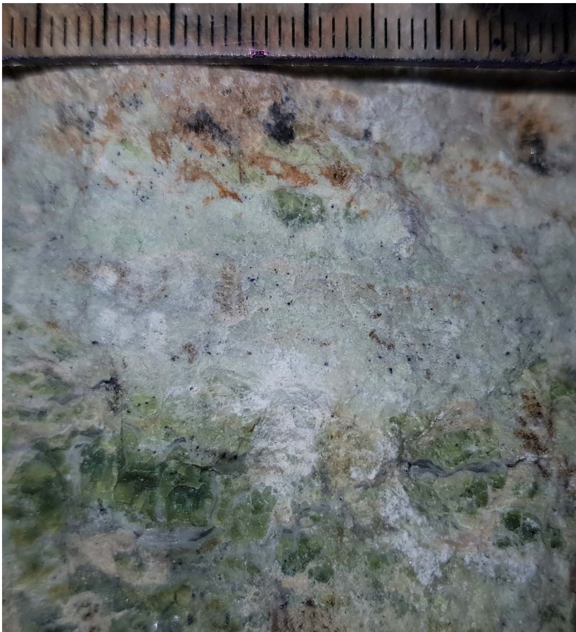
Photograph 5: Calcrete from MG1 Apron, Sample 8 (Scale in mm).
