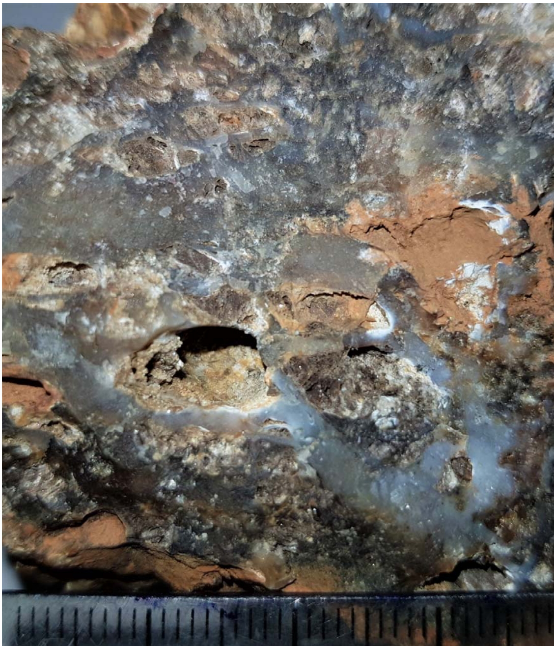
Photograph 7: Silcretised ultramafic, Sample 7 (Scale mm).
