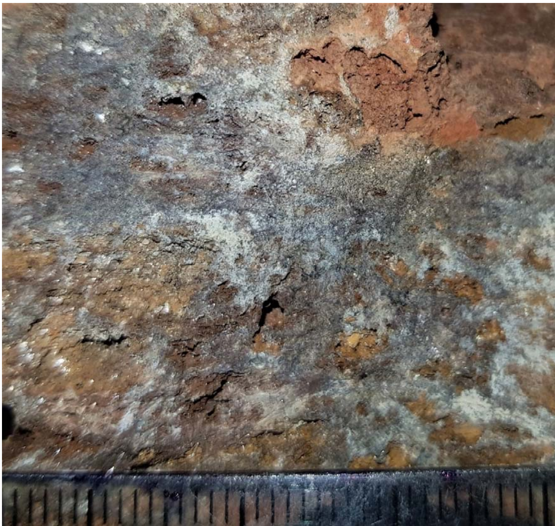
Photograph 6: Silcretised ultramafic, Sample 7 (Scale mm).
