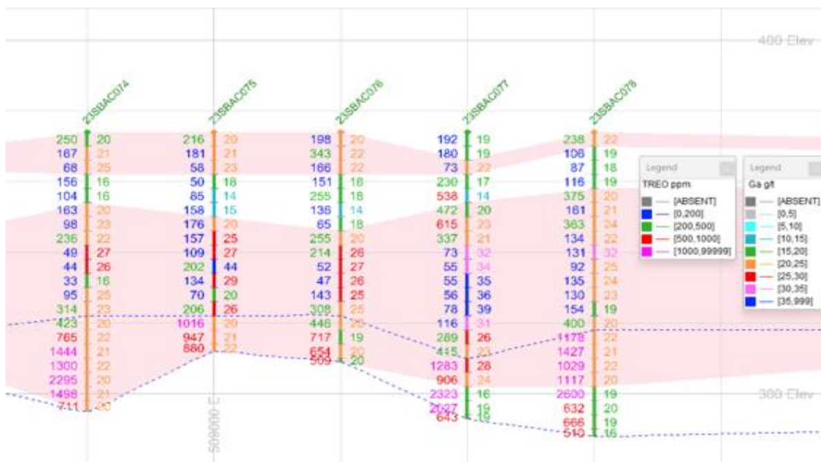
Diagram: 7 (Drill section line 6,765,800mN) – Mineral grades highlighted above show that Gallium mostly sits above the REE zones which also contain Gallium; Left hand side REE with Gallium grades on the Right-hand side of the above drill collars. Areas indicated in pink indicative the +20g/t zones of Gallium sitting in clays/Oxide. The blue dotted lines highlighting the elevated REE and Gallium sitting along the hard rock interface zone (no drilling data into the underlying hard rock).
