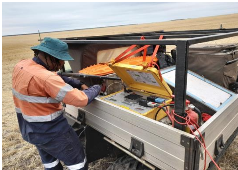
Picture 2. Ground EM survey at Lort River Project. Above picture shows the UTV charging station and one of the two EM survey operators, (other team member of the three positions cables) who is located at one corner of the actual on ground wire loop (8m or 10mm copper cable), the cables are laid out on the ground in a large 200m square loop. The above vehicle (UTV) has a charging station (yellow control box and battery).
