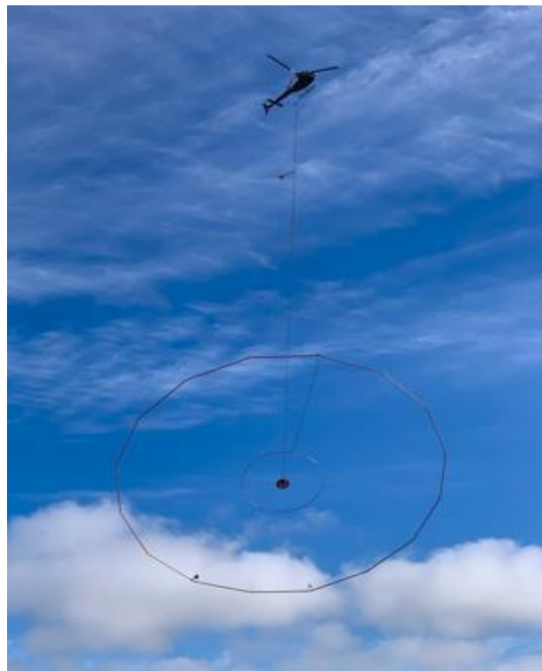
Picture 1: Helicopter with VTEM survey sensor array over the 100% owned Lort River Project.
