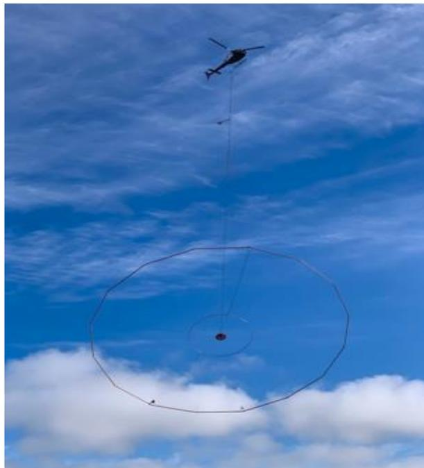
**Picture 1:** Helicopter with VTEM survey sensor array.
