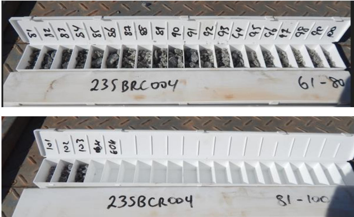
Picture 2. Chip tray showing 1m RC drilling samples, each box is representative of a ~1 meter interval in hole 235BRC004 from the Smokebush pegmatite drilling campaign.
