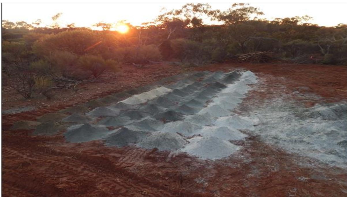
Picture 3. Drill spoil material, showing the contrast between basalts and other mafics and ultramafics and the white spoils piles indicating intervals of interpreted pegmatite, hole 235BRC004 at Smokebush.
