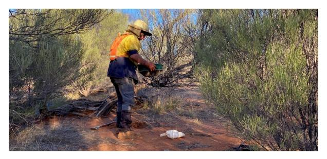
**Picture A:** XM Logistics team member at Larins Lane. The soil sampling program utilised the mobile metal ion (or MMI) soil sampling technique (Note: all sample collection tooling is plastic).
