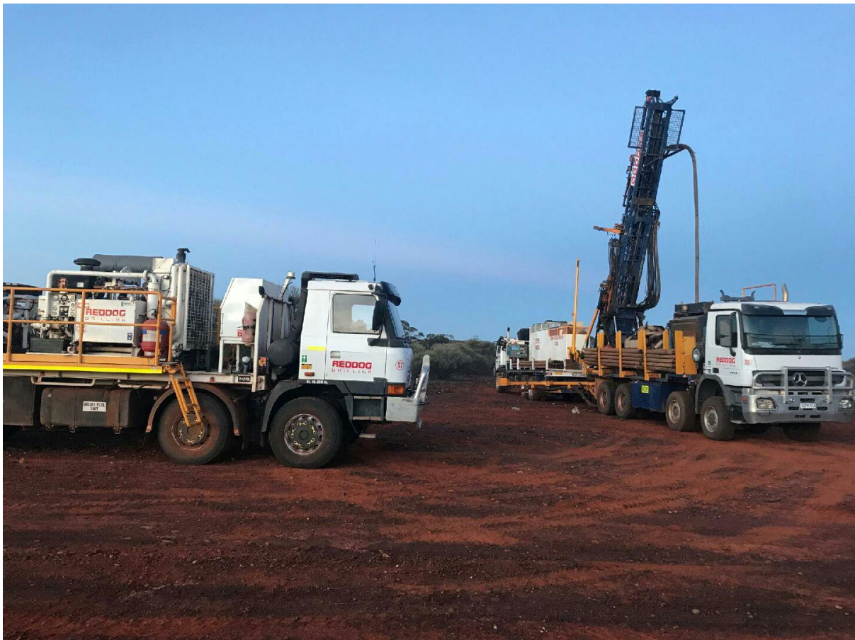
Picture 1: The RedDog Drilling set up for the first hole at Monza - Smokebush Gold Project.
