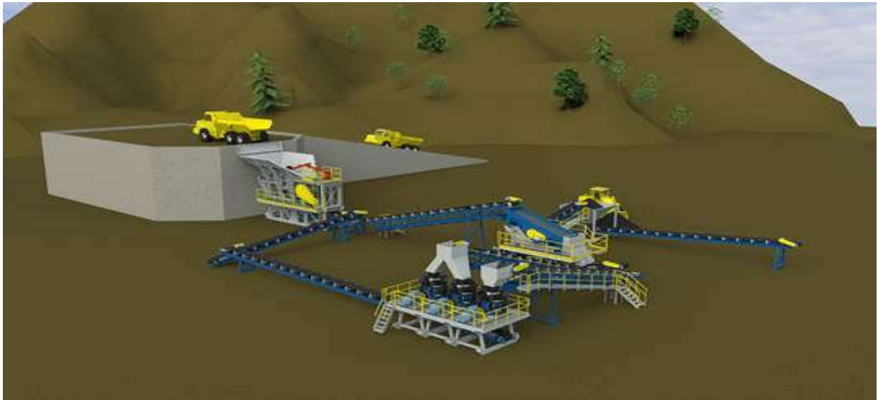
Diagram 1: Sepro Systems 75t/h three stage crushing circuit.
