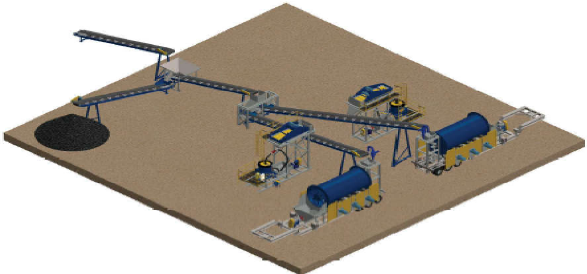
Diagram 2: Sepro Systems 40 tph grinding and gravity plant (dual stream mills and centrifugal concentrators).
