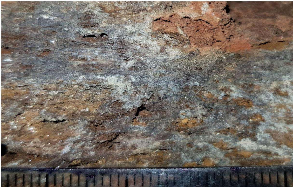
**Picture 7:** Silcretised Ultramafic, Sample 7 (Scale mm).
