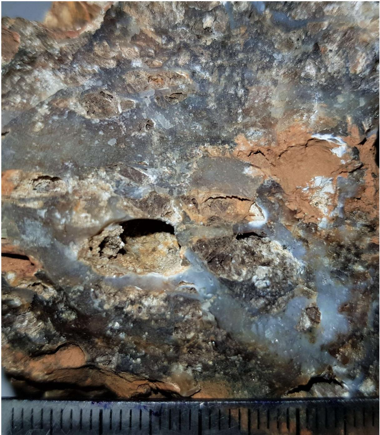
**Picture 8:** Silcretised Ultramafic, Sample 7 (Scale mm).
