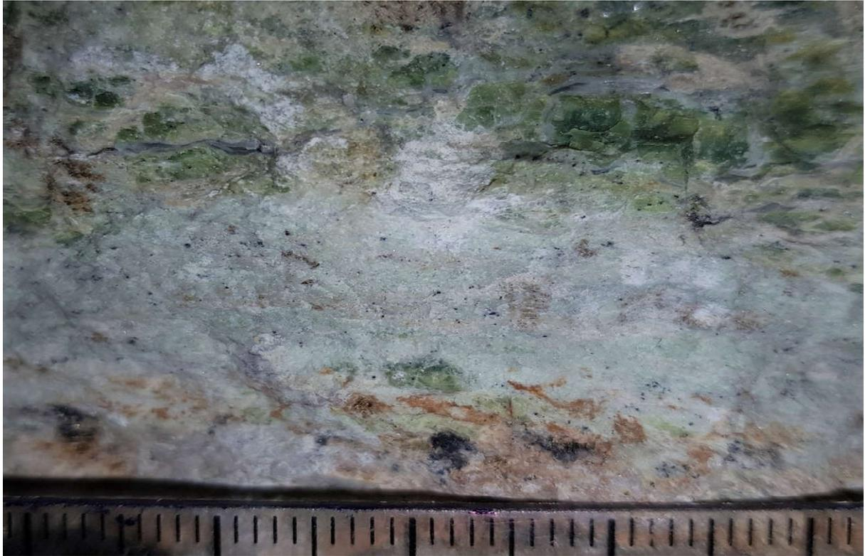
**Picture 6:** Calcrete from MG1 Apron, Sample 8 (Scale in mm).
