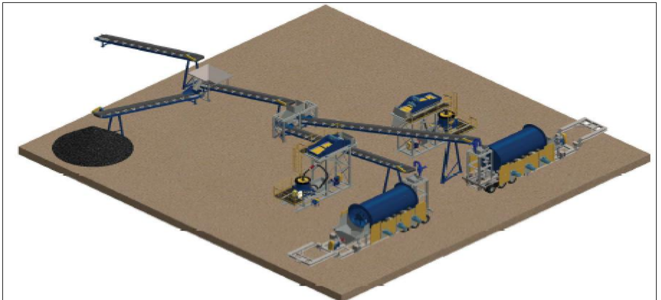
Figure 6: Sepro Systems 40 tph grinding and gravity plant (dual stream mills and centrifugal
