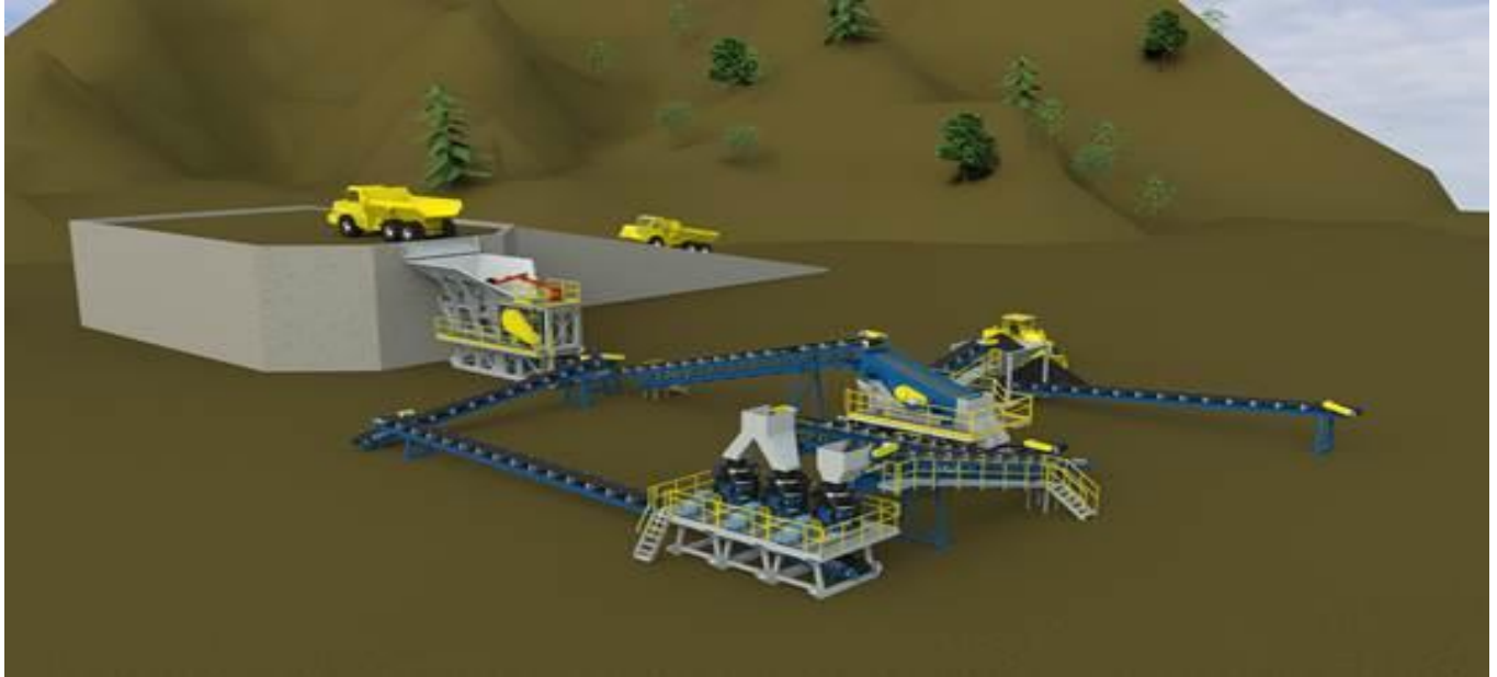
Figure 5: Sepro Systems 75t/h three stage crushing circuit
